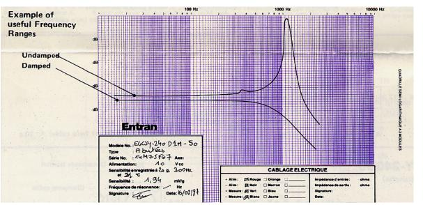
• Typical real accelerometer frequency response.
